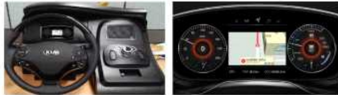
Fig. 18. Automotive digital cluster hardware and display.
