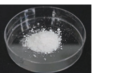
Sulfate esterified cellulose nanofiber in powder form
